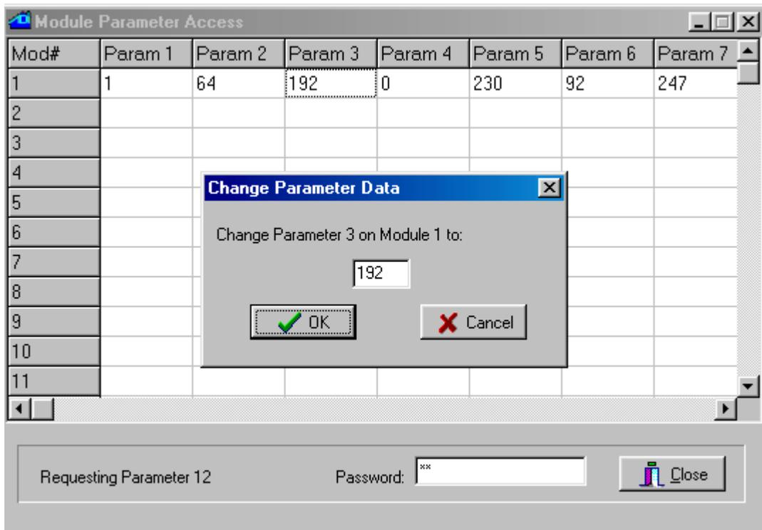
The threshold values can also be used to perform reverse logic. Lets say for example you want an input to be OFF when closed and ON when open, such as a door sensor in a security system. This can be done by setting the low threshold to 0 and the high threshold to 128. If you wanted to have the input report OFF when open and ON when closed, set the low threshold to 128 and the high threshold to 255. This can be done with analog or supervised inputs.
