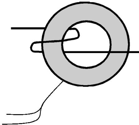
For beds that pull less than 10 AMPS, wrap the wire around the T-Max® Sentry™ one time.
