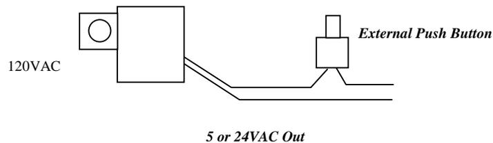
The T-Max® 3A can be ordered with an external push button option. When 5 or 12Volts is applied to the External Start input on the T-Max® 3A while it is in Delay, the bed will be energized with out having to press the Start/Stop button. Above is an example of an push button circuit.
